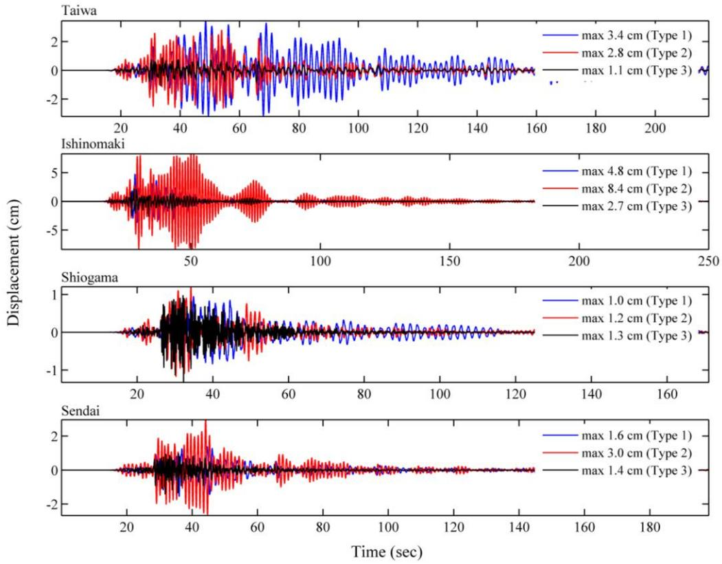
Fig. 8 Top displacement records of three type structure at four stations
