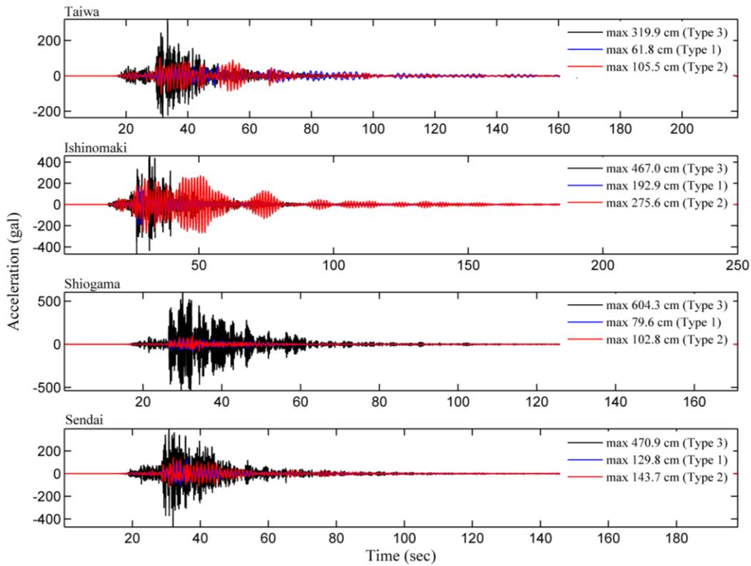
Fig. 9 Top acceleration records of three type structure at four stations
