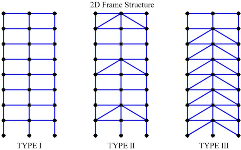
Fig. 5 Modeled frame structure with three stiffness type
