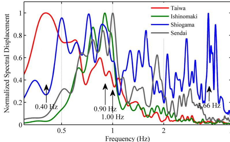
Fig. 7 Displacement frequency content of August 16, 2005 earthquake
