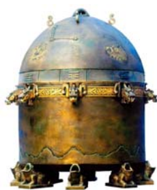
Fig. 3 Reconstruction designs based on a suspended pendulum
